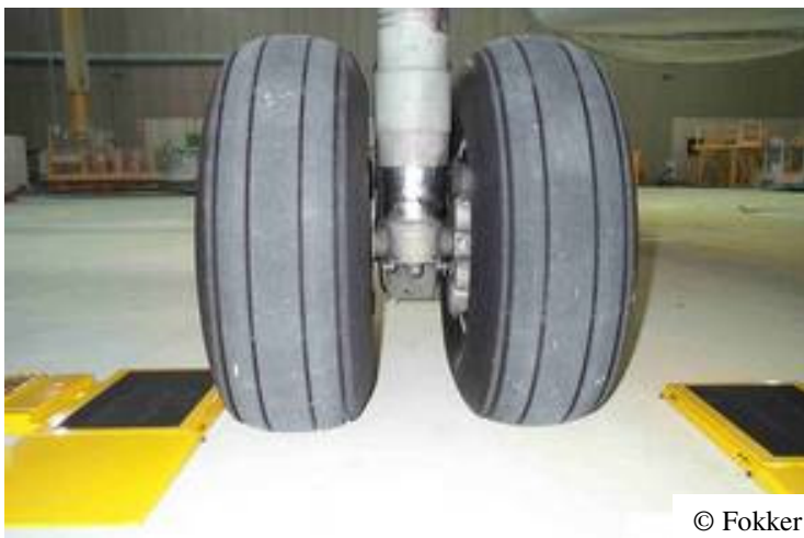
Figure 6: Weighing of Fokker 70 Nose and Main Landing Gear Platform
